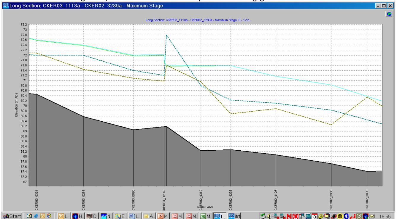
Figure 8) Long-section 100 year water levels. Green line = original cross-section, blue line = new shoal.
