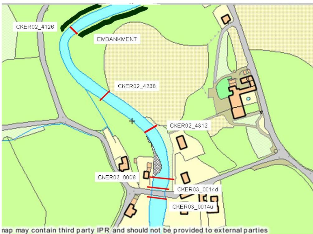
Figure 1) Cross –section layout showing shoal below bridge and embankments.
