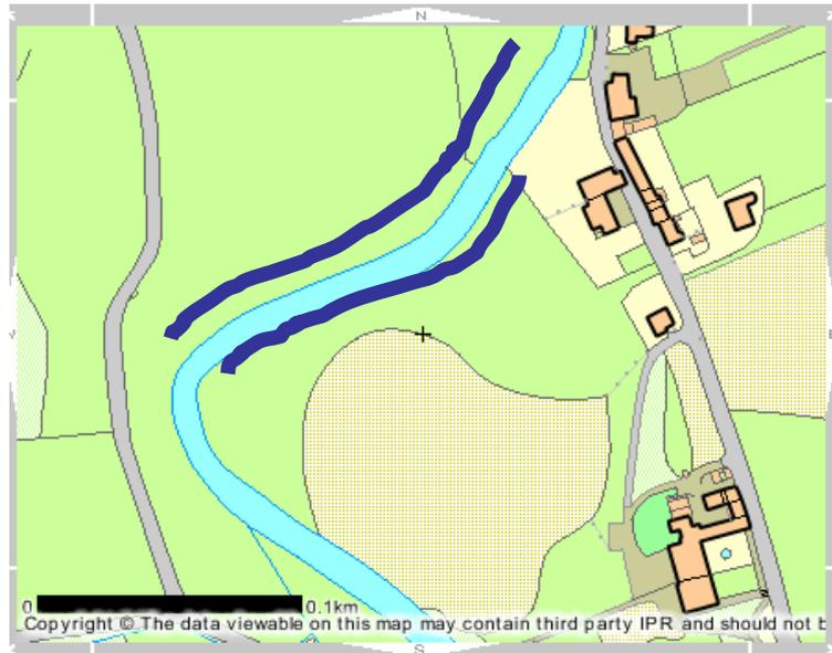
Figure 4) Embankments to be removed.
