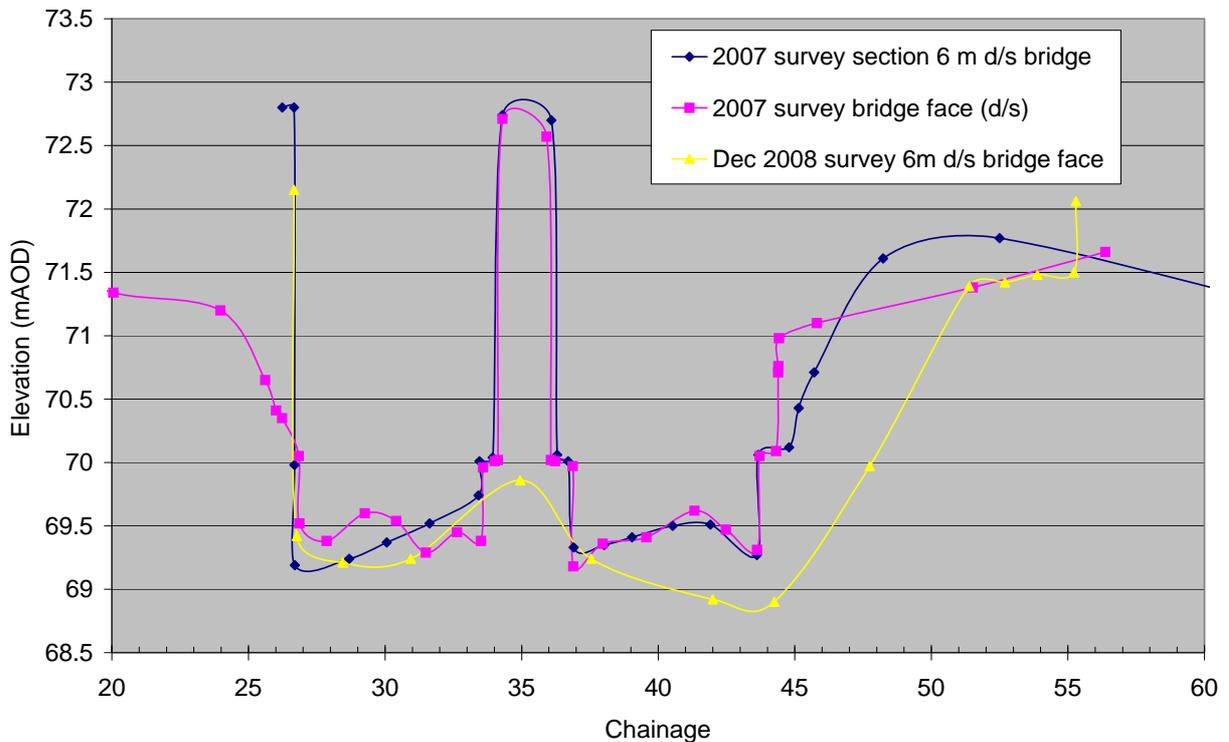
Figure 5) Cross-section survey below the bridge –blue and pink are 2007, yellow is the Dec 2008 survey.
