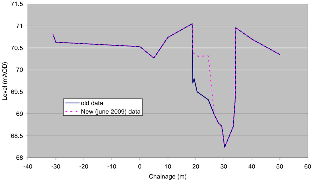
Figure 10) Cross-section taken in June 2009 through the shoal
