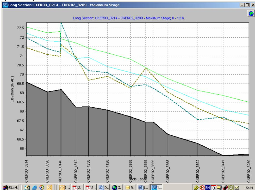
Figure 3) 1% AEP, maximum levels at Low Lorton, Green = Full embankment scenario, Blue = no embankments. (Cocker03\_0014u is the bridge)
