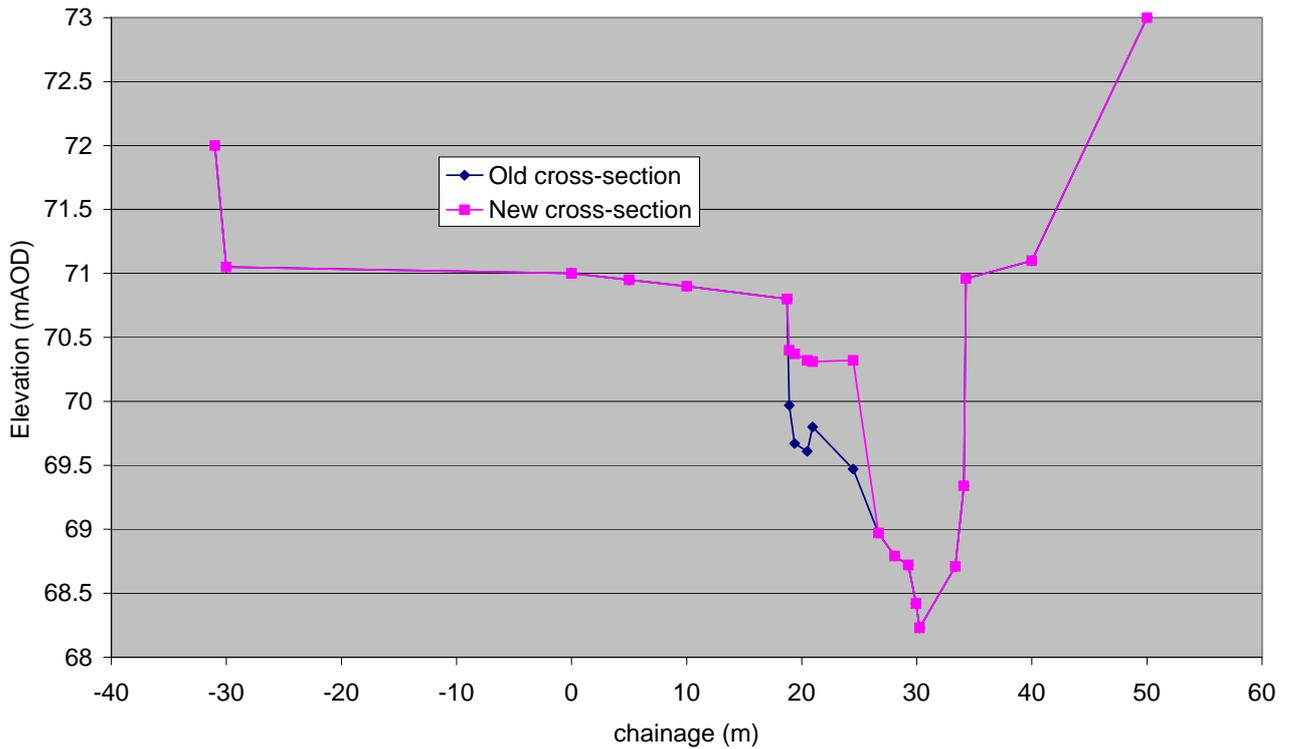
Figure 7) Revised cross-section profile showing gravel shoal.
